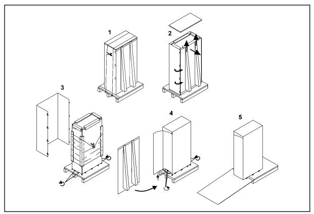
Figure 3 Unloading the equipment from the pallet.
